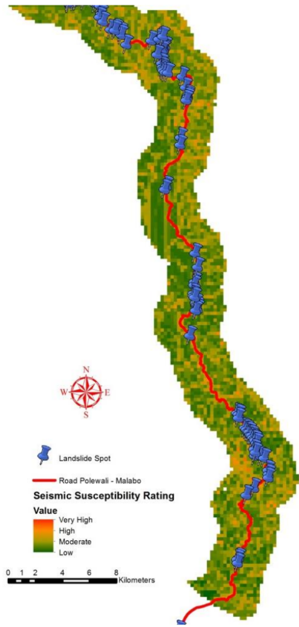
Figure 11. Landslide spots were observed in the conducted field survey.
